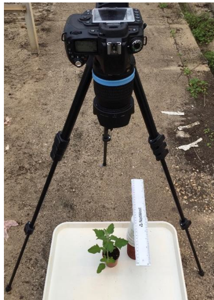
Figure 2. Method for taking photographs for leaf area determination. An untreated Chenopodium album seedling is shown, 3 weeks after the application of glyphosate treatments using a Nikon D90 Digital SLR Camera with 18-105 mm VR Lens Kit and a Manfrotto Compact Action tripod. Ruler was set at the height of the seedling in order to calibrate the WinDias software.
